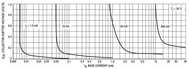
Figure 4. Collector Saturation Region
